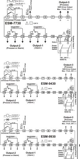
Note-1: There is an internal fusible flameproof resistor. Note-2 : External fuse is recommended
